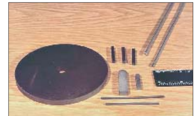
Rod and disc electrodes for PED and TRESS
