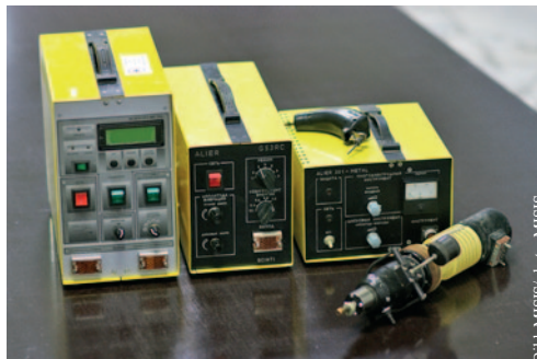
Abb. 6: Niederspannungs-Hochfrequenz Anlage für PED Fig. 6: Low-voltage high-frequency equipment for PED
